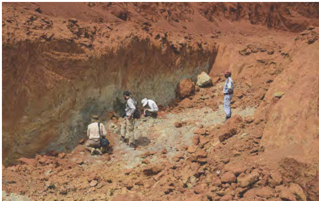
Figure 5. Left: A clear contact between the topsoil and the ruby-containing amphibolite can be found on the walls of the primary deposit pit. Photo by Andrew Lucas/GIA. Right: The top of the ruby-containing layer has been extensively weathered, and the rock is very fragile. Photo by Vincent Pardieu/GIA.
