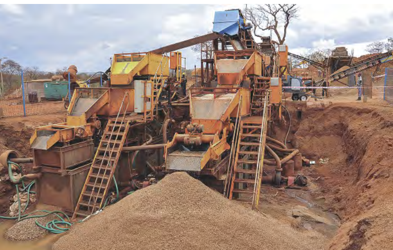
Figure 16. Two sluices, or jigs, are used for different-sized gravel. The heavier material is trapped in the grooves of the jig, while other material goes into the piles in front. Photo by Vincent Pardieu/GIA.
