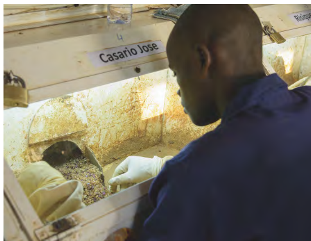
Figure 17. The first step of sorting is to separate ruby and garnet from the washed gravel. Sorters do not touch the gravels with their hands. Instead, they wear rubber gloves attached to cloth sleeves. Photo by Andrew Lucas/GIA.
