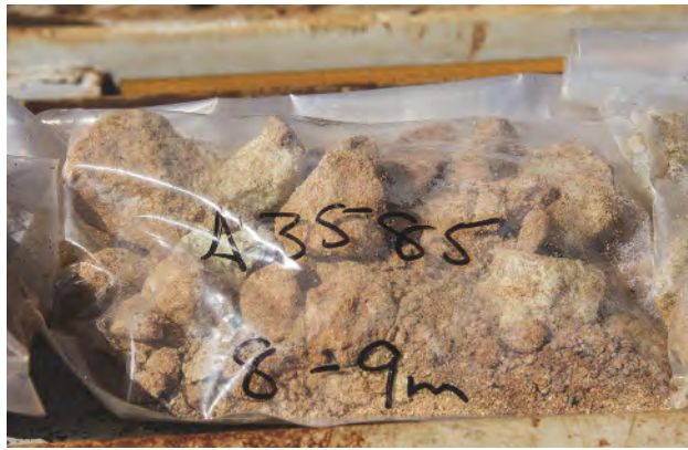
Figure 11. The soil and the gravel are sampled at every meter until the drill strikes bedrock. The machine will continue another meter or two to finish the sampling. Photo by Andrew Lucas/GIA.
