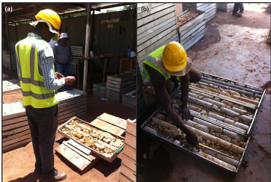
Figure 3-5: Geo-assistant core photography (a) and core mark up (b) observed during the March 2015 SRK site visit
