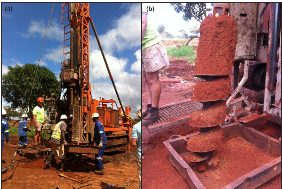
Figure 3-6: Auger drilling at Mugloto observed during the March 2015 SRK site visit, a specially modified Sandvik DE700 diamond rig (a) with an auger drill bit (b)
