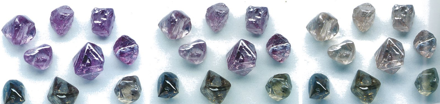
Figure 2. The colour of pink diamonds can be deepened (left) or lightened (right) and returned to their original 'daylight' colour (centre) after illumination with white or blue light. The brown diamonds are for colour reference.
