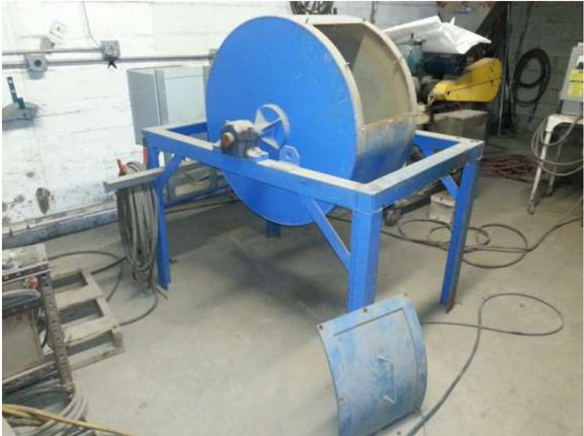
Figure 13.5 FLS Tumble or breakage test unit (modified ASTM Test E279)
