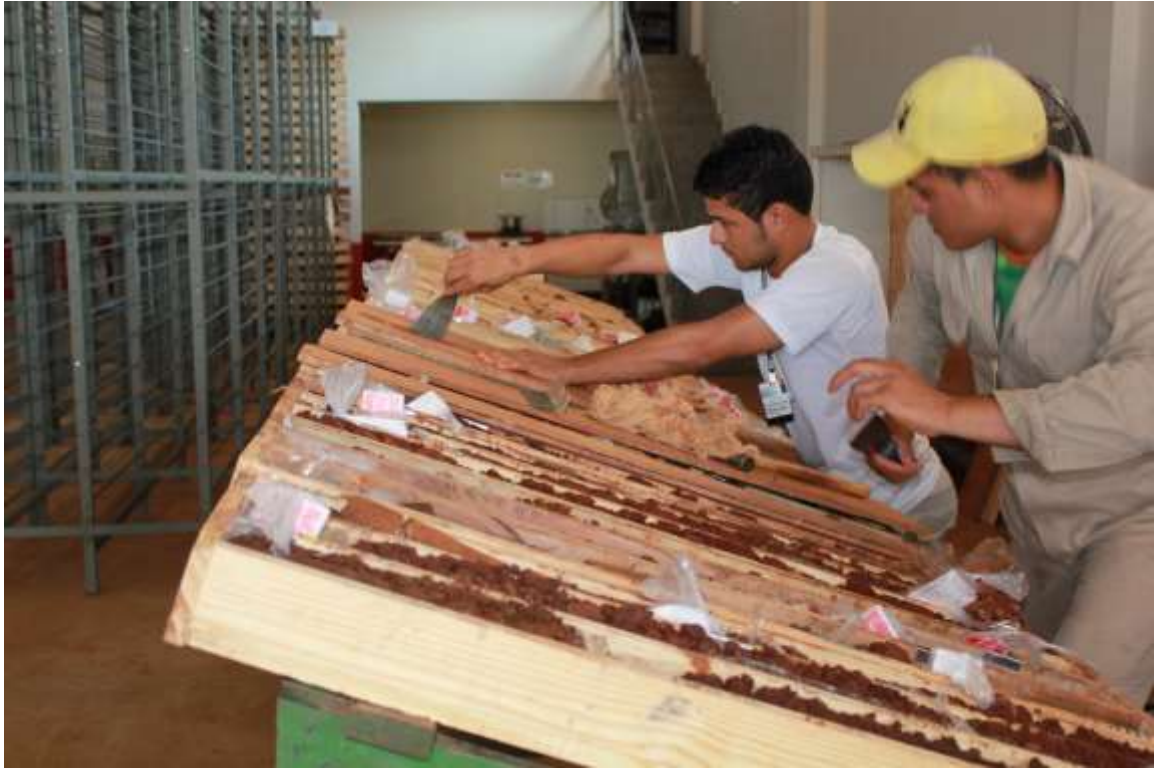
Figure 11.2 Splitting soft core with paint scraper
