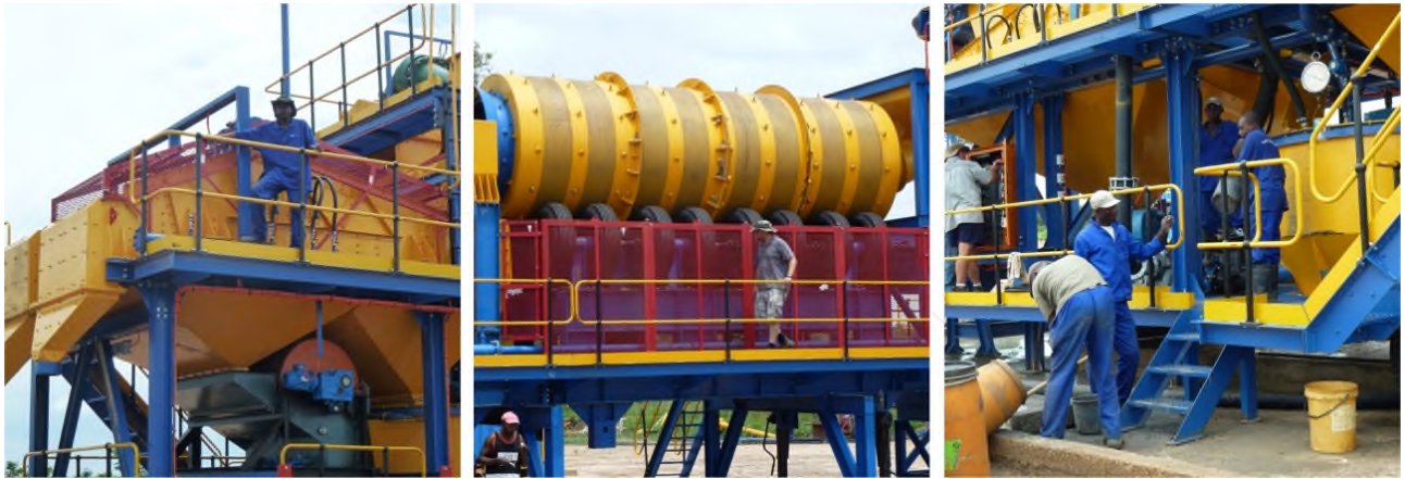
Lucapa's 150 tonne per hour diamond plant at Lulo
