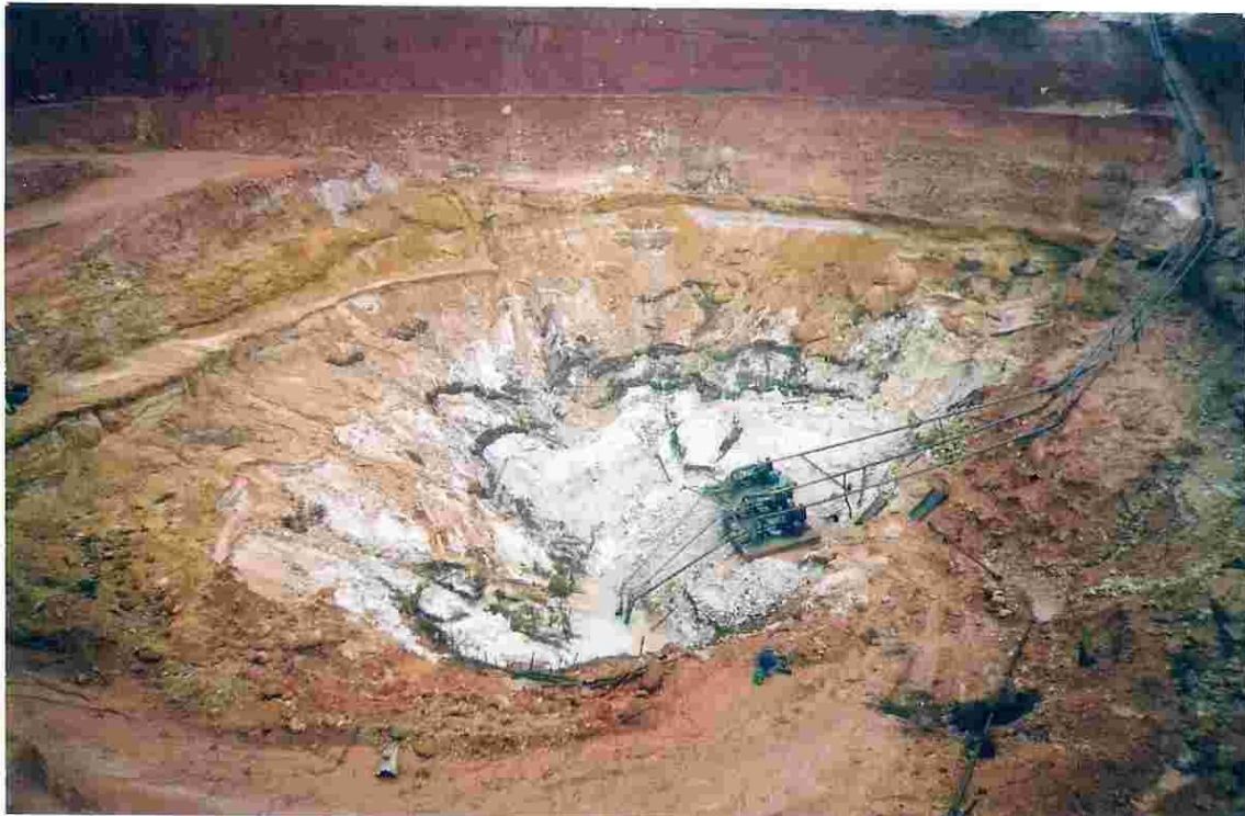
Figure (28): Slumping, in places, of the Pit walls despite the insertion of lines of timber stakes. Three gravel pumps are visible, situated on bedrock.
