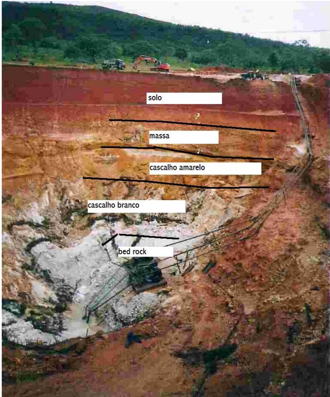
Figure (14): Stratigraphic succession on the Property 15 . From the surface: soil (solo), massa, yellow gravels (cascalho amarelo), white gravels (cascalho branco), and quartzitic bedrock.
