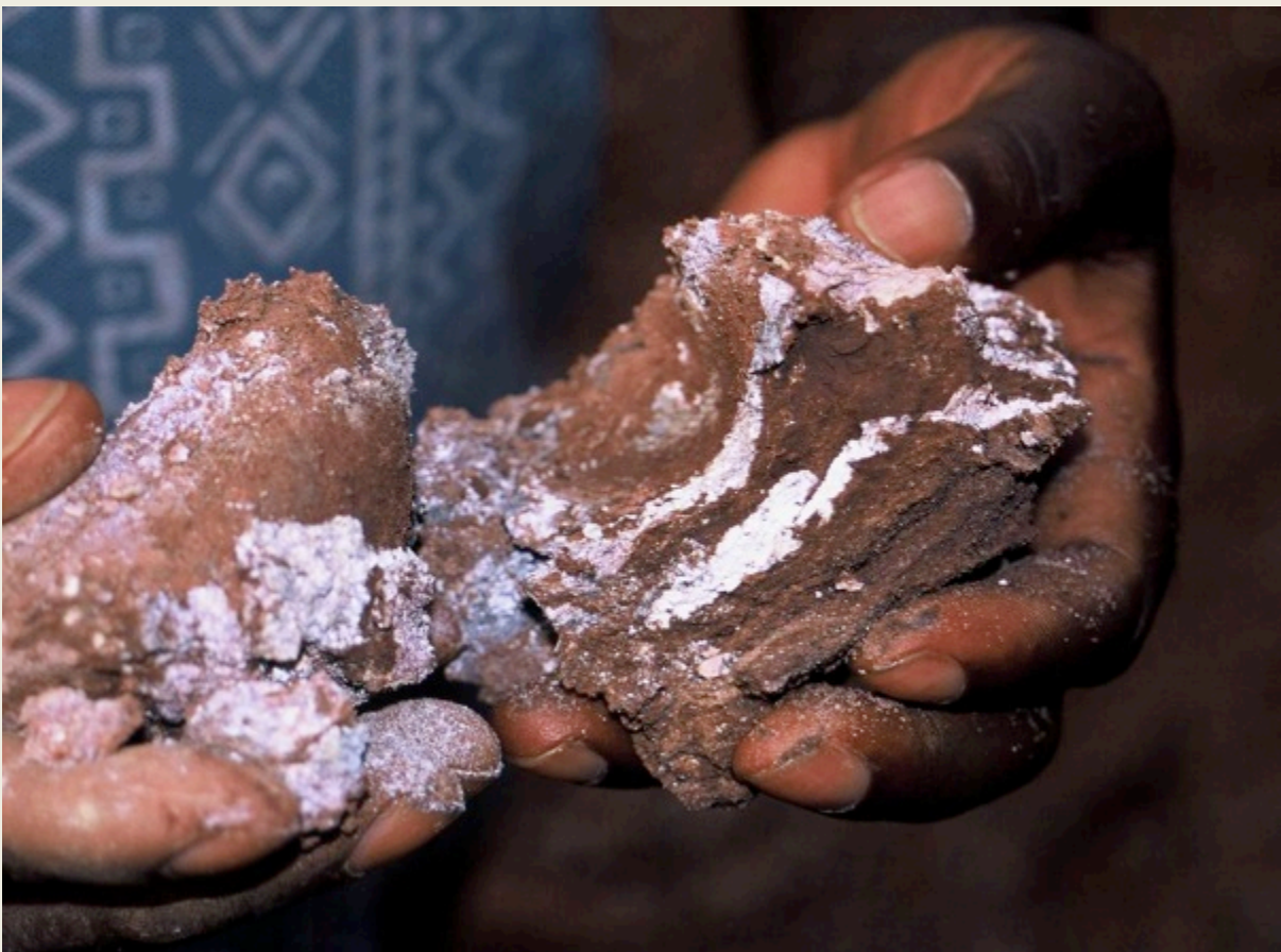
Figure 64 - A sample of typical Calonda Formation basal conglomerate.
