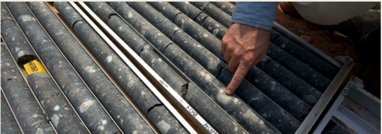
Figure 32 - Kimberlite core recovered from new discovery in the Tchegi area.
