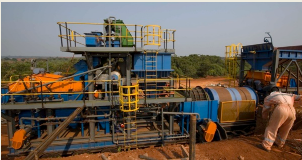
Figure 30 - Exploration treatment plant in the left margin of the Chicapa River - Itengo area.
