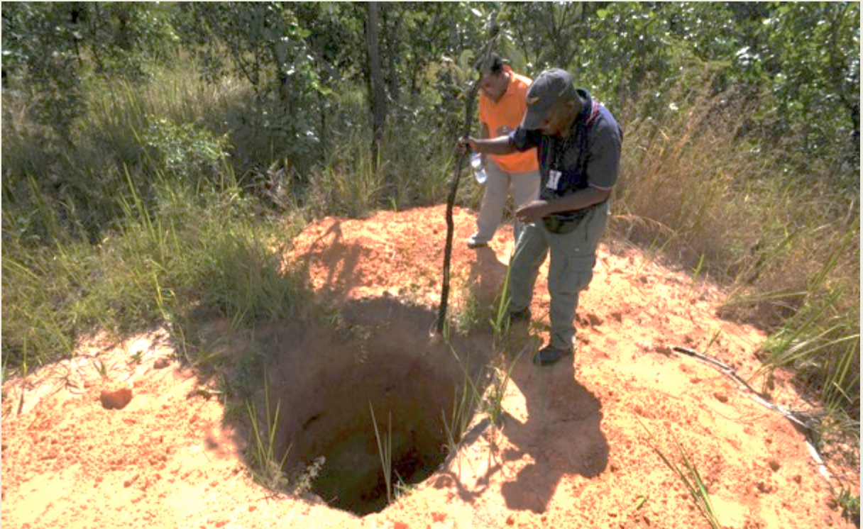
Figure 41 – An abandoned garimpeiro exploration well ( poço zairese ) – S Malanje province.
