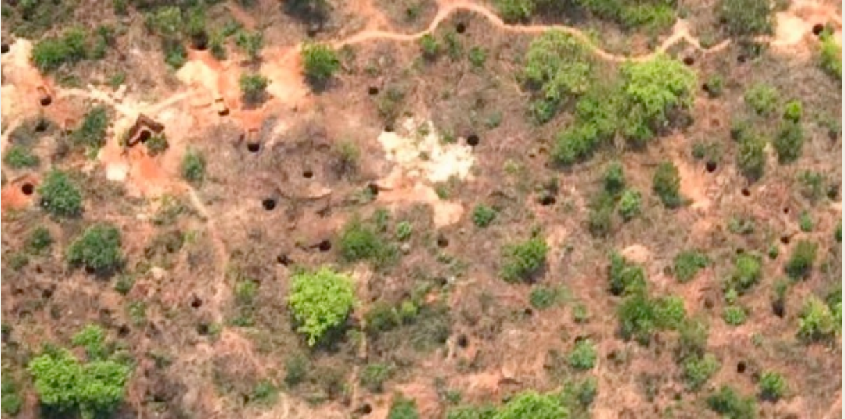
Figure 40 - Swiss cheese scenario generated by garimpo (vertical wells connecting underground tunnels) over a likely kimberlite – Tchegi area.
